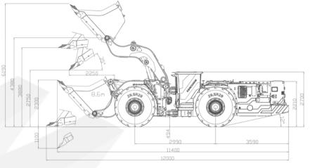
Length: 11 Width: 3 Height: 2 Total weight: 46 Standard bucket: 8, Tramming capacity: 17 Power rating: 33 Exhaust gas purity class: St
