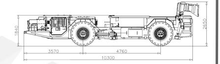
Length: 10 300 mm Width: 3 440 mm Height: 1 900/2 000 Total weight: 26 320 kg Standard box volume: 11,1 m Nominal Rated Payload: 20 Mg Power rating: 168 kW Exhaust gas purity class: Stage V
